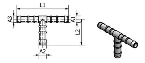
Ext. Hose Diameter A3 = 5 Ext. Hose Diameter A1 = 5 Ext. Hose Diameter A2 = 5 L1 = 42 L2 = 22
